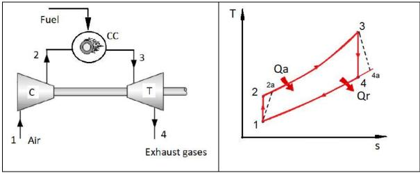
The above figures represent flow and T-s diagrams for the gas turbine unit.
