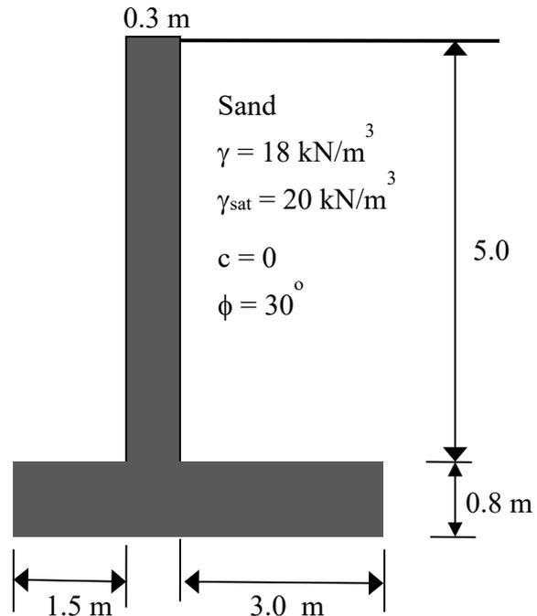
the earth pressure,  $P_a = k_a \gamma H = 0.33 \times 18 \times 5.8 = 34.45 \text{ kN/m}^2$
