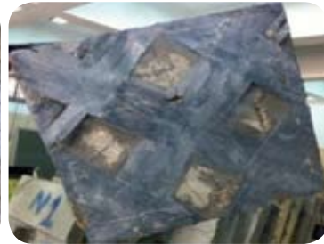
Fig. 5 – Rupture of CFRP at S6
