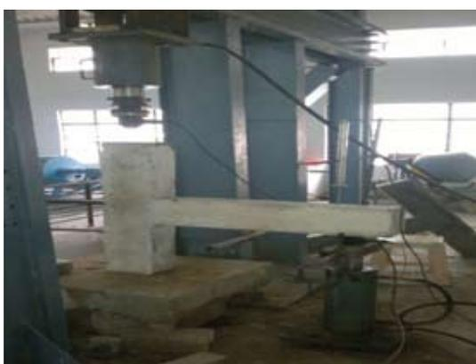
Specimens were tested in a universal testing machine of 294.3 KN (or 30 t) capacity. A constant load of 15.7 KN (or 1.6 t), which is about 20% of the axial capacity of the column,
