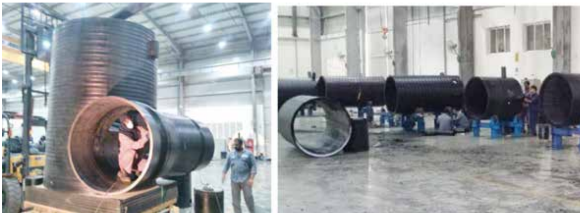
Picture 3- Manufacturing of Manholes
