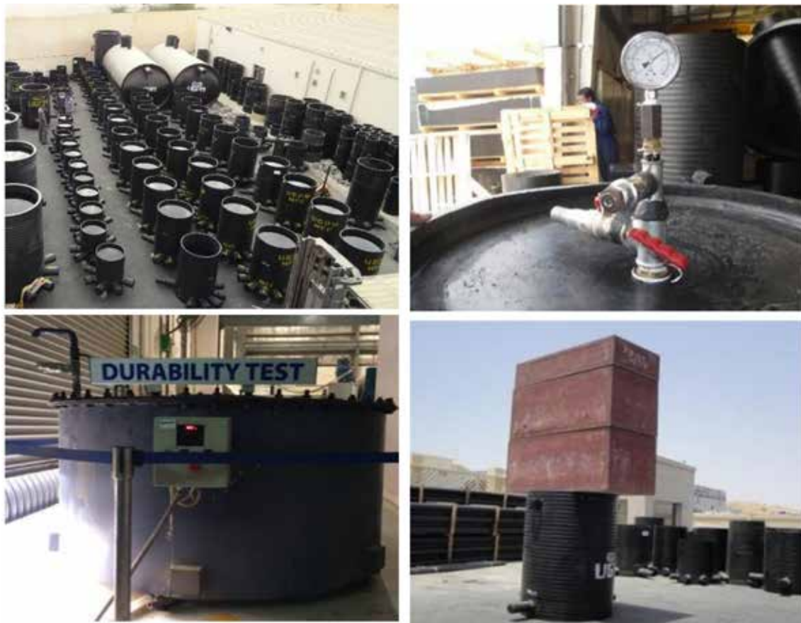
Picture 4 – Quality control test on final product. Top left – Leakage test, Top Right – Vacuum Test, Bottom Left – Durability test, Bottom Right – Load Bearing test
