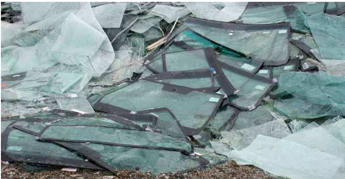
Figure 1: Laminated windshields are difficult to recycle using standard methods because it contains layers of glass and plastic. Image adapted from: Ildar Sagdejev; CC BY-SA 4.0
